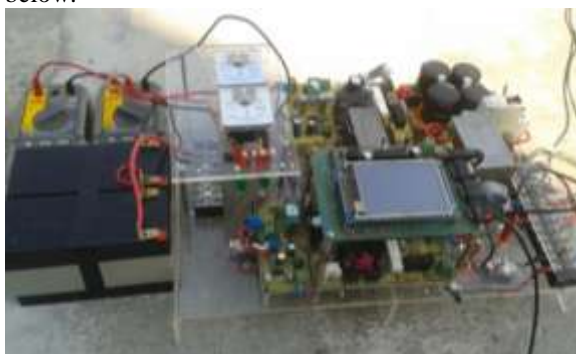
Figure 10. Prototype of parallel boost for battery charging The result of tested OS task priority on handling control algorithm can be seen on Table 5 below.
